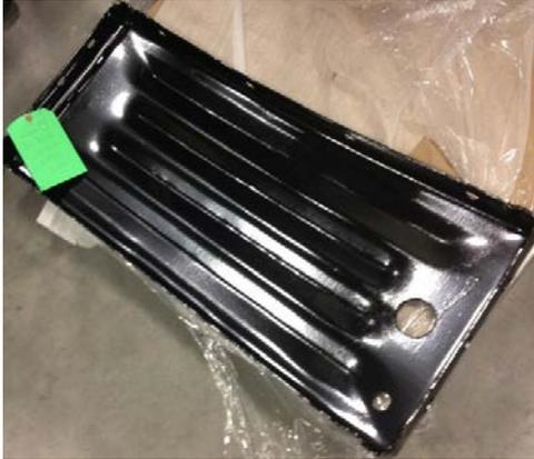
**Figure 4: Typical Polymer Coated Liner Plate**
