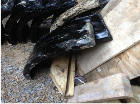
**Figure 3: Typical Galvanized and Bituminous Coated Liner Plate**
