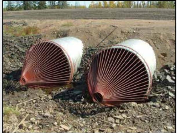
CONICAL GRATES WITH FISH OPENING (PATENTED DESIGN)
