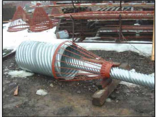
CONICAL GRATE WITH PERFORATED CSP
