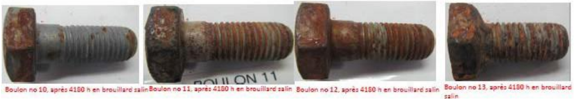
Photo no 2: After 4,180 hours of Salt Spray Test
