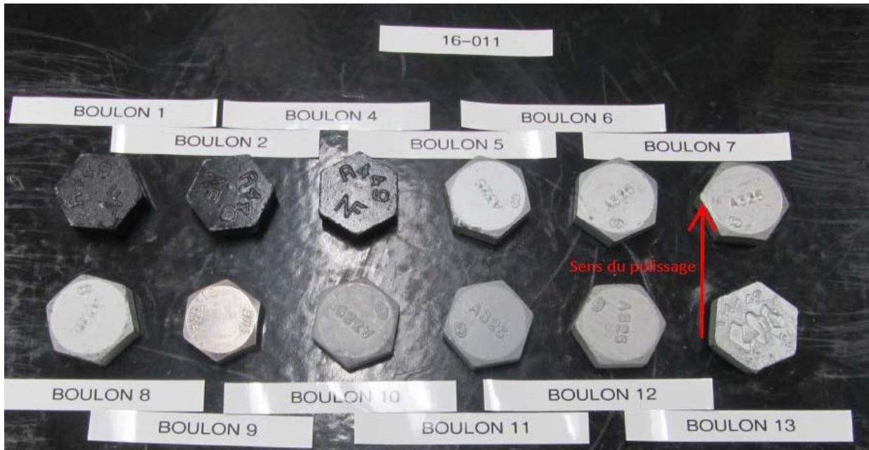
Photo no1: Arrangement of samples for the abrasion test
