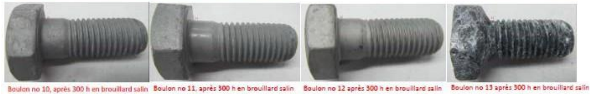
Photo no1: After 300 hours of Salt Spray Test
