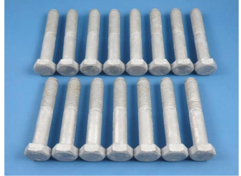
After 9 cycles Volvo ACT II test
