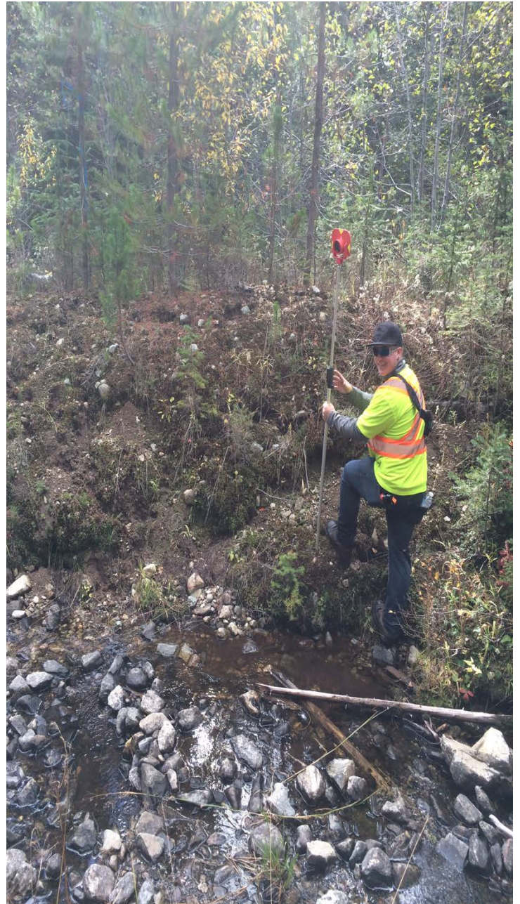
Fig. 5 – Upstream Debris Loading and High Water Mark (Taken by Eric)
