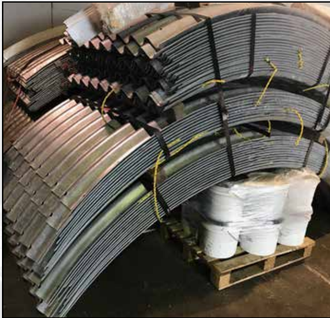
FIGURE 3 - WAREHOUSE STORAGE/PLATE STACKED WITH POLY ROPE SPACERS
