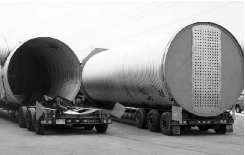
Detention tank with internal baffle for sediment and debris control. (Ministry of Transportation, Ontario)
