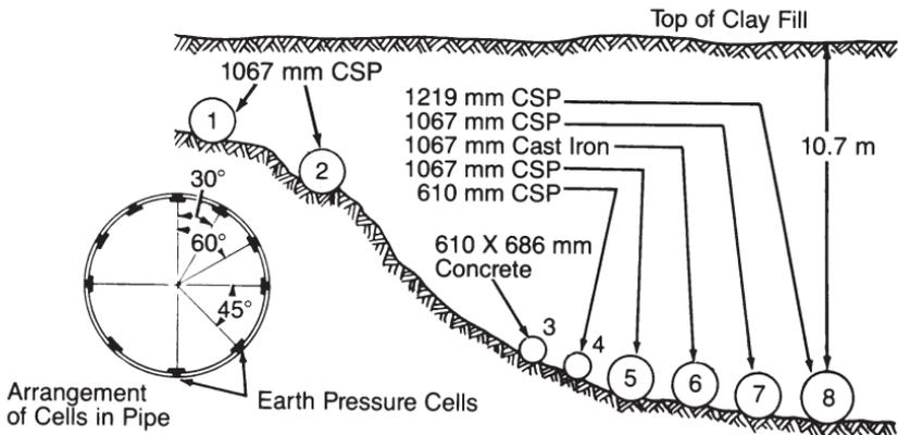
**Figure 6.1** American Railway Engineering Association tests on culvert pipe.
