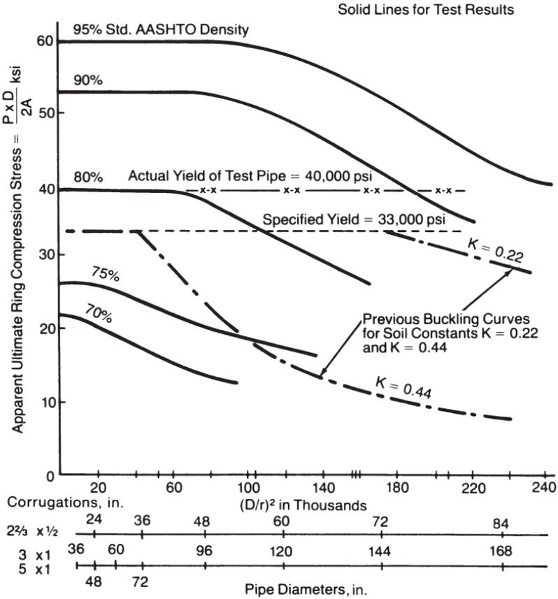
**Figure 6.30** Results of Utah loading tests on corrugated steel pipe, showing apparent ultimate ring compression stress as a function of diameter and corrugations for various values of soil density determined by AASHTO.
