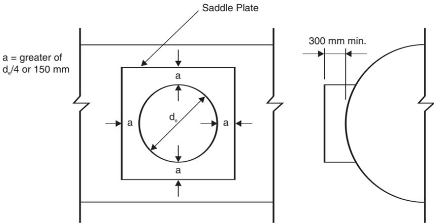
**Figure 6.20** Schematic of saddle plates.
