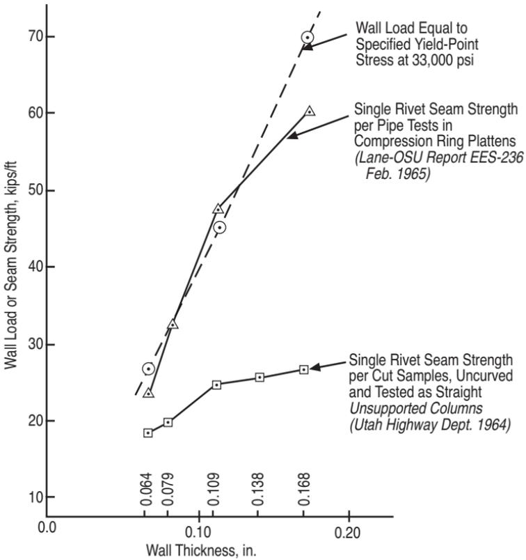
**Figure 6.32** Comparison of single-rieveted seams tested as straight, unsupported columns by Utah and those tested in compression ring patterns (comparable to actual service) by Ohio. Pipe seams have no apparent effect on the strength of the pipe.
