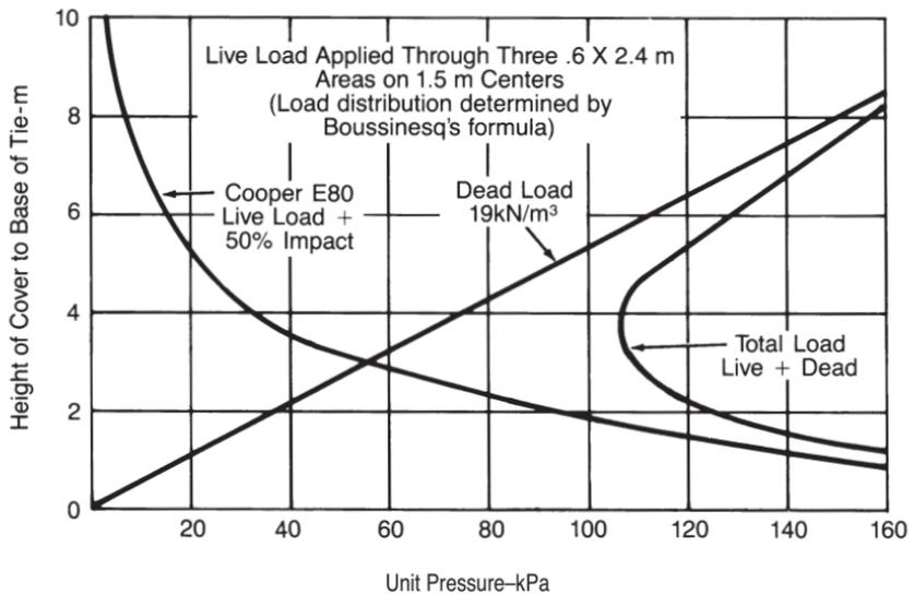
**Figure 6.4** Combined E80 railway live load and dead load.
