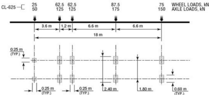
Position as many axles of the CL-625 truck within the span length, ( $D_h = 9.006$  m), at the road surface as would give the maximum total load. In this example, placing axles 2, 3, and 4 above the structure produces the highest total load ( $P = 425$  kN)
