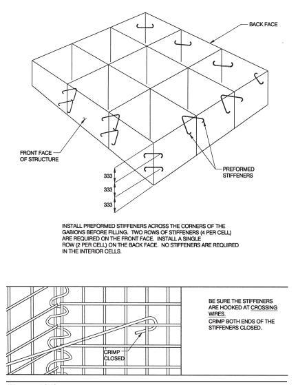
Figure 13.8 Welded wire gabions preassembly.
