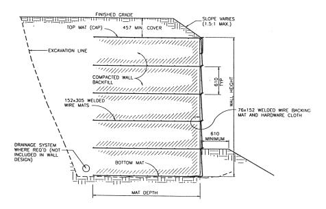
Figure 13.4 Welded wire wall.
