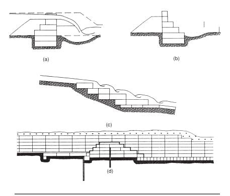
Figure 13.6 Typical gabion weir cross sections: a) vertical face; b) stepped face; c) long stepped; and d) sloped.
