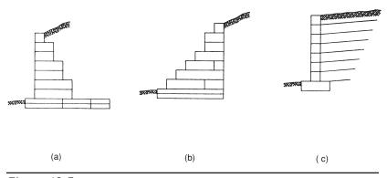
Figure 13.5 Typical cross sections for a) gravity gabion wall (stepped); b) semi-gravity gabion wall; and c) reinforced soil gabion wall.
